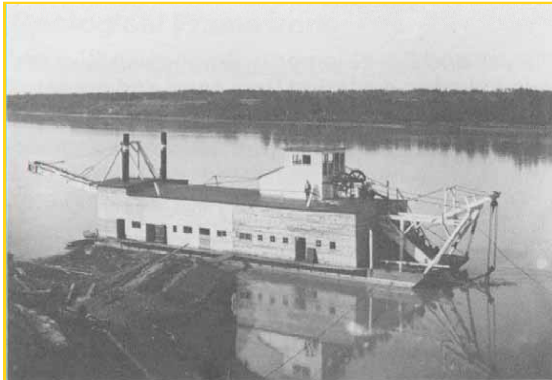
Plate II. Large dredge with frame superstructure, North Saskatchewan River, 1905 (Photograph courtesy of Saskatchewan Archives)
